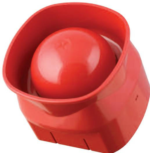
The Symphoni Voice+ is an ultra-low current sounder that can be supplied with up to 16 voice messages. Normally the unit is loaded with 3 commonly used messages. The sounder also has international tones available and a user selectable setting so that messages can be played without the use of a tone.
